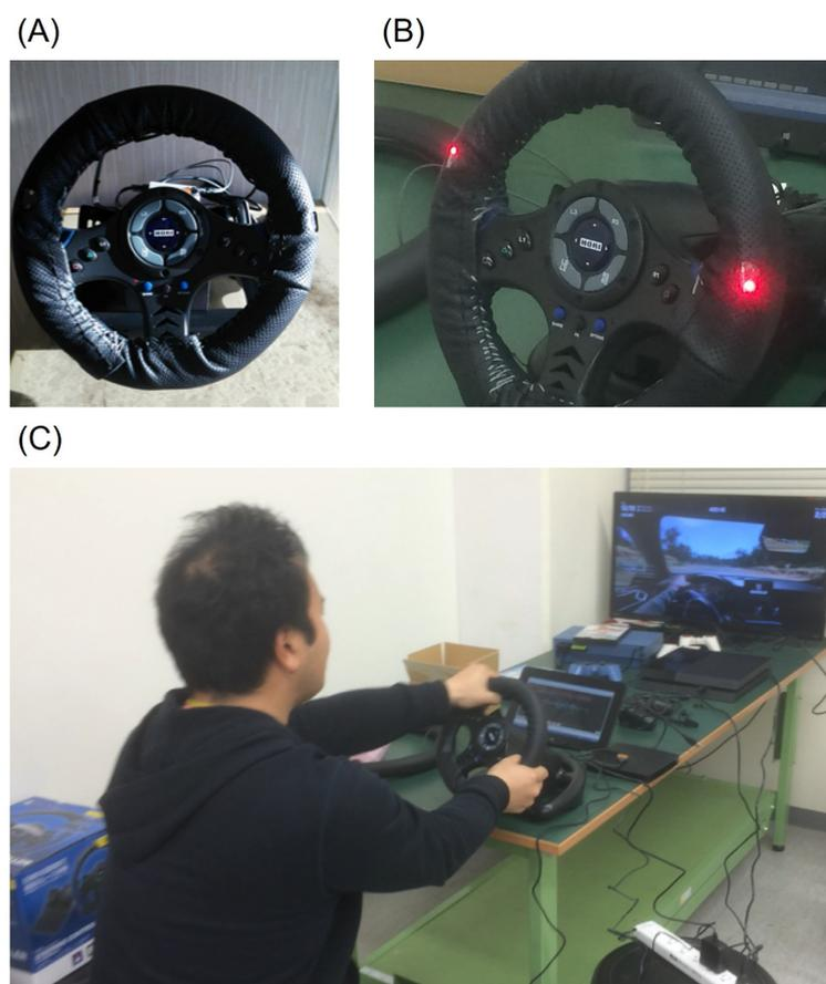
**Figure 2.** Steering-type measurement system developed by Arakawa et al.: (A) appearance of the system; (B) transmitter and receiver LEDs visible on the spoke of the steering wheel; (C) demonstration of the operation of the system while playing a driving game.
