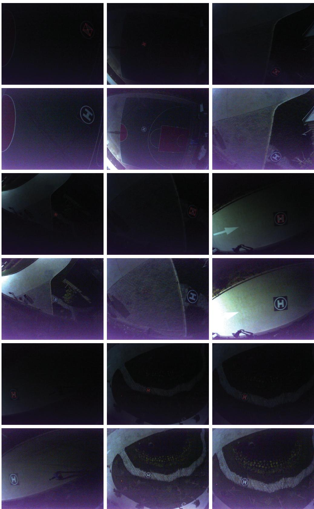
**Figure 10.** The landing marker detection results of the proposed vision system. The first, third, and fifth rows: Selected color images from the original test dataset. Detected markers are highlighted in color lines and dots. The second, fourth, and sixth rows: The corresponding color images after enhancement for scene detail observation.
