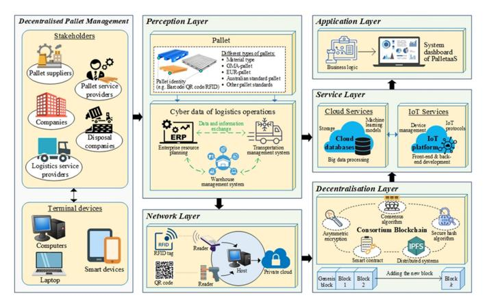
Figure 2. Layered architecture of PalletaaS for the decentralised pallet management.
