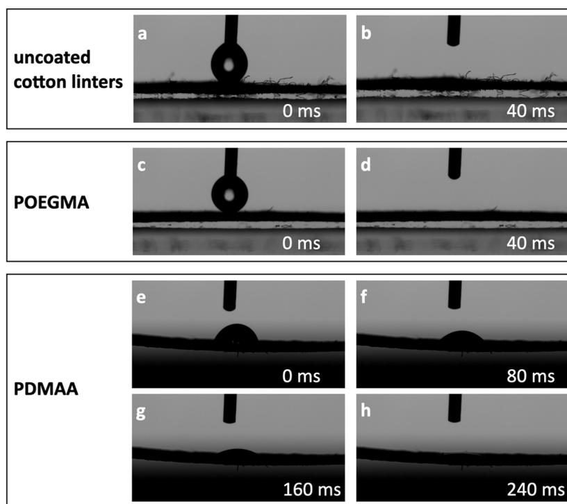
**Figure 3.** Dynamic water contact angle changes on uncoated (a,b), POEGMA-coated (c,d), and PDMAA-coated (e–h) cotton linter paper. A 2  $\mu$ L drop of water is applied to the paper, and the time until full imbibition is measured. The total imbibition time for the PDMAA experiment was 7 frames (280 ms), and, for the POEGMA-coated and uncoated paper, less than 1 frame (40 ms).
