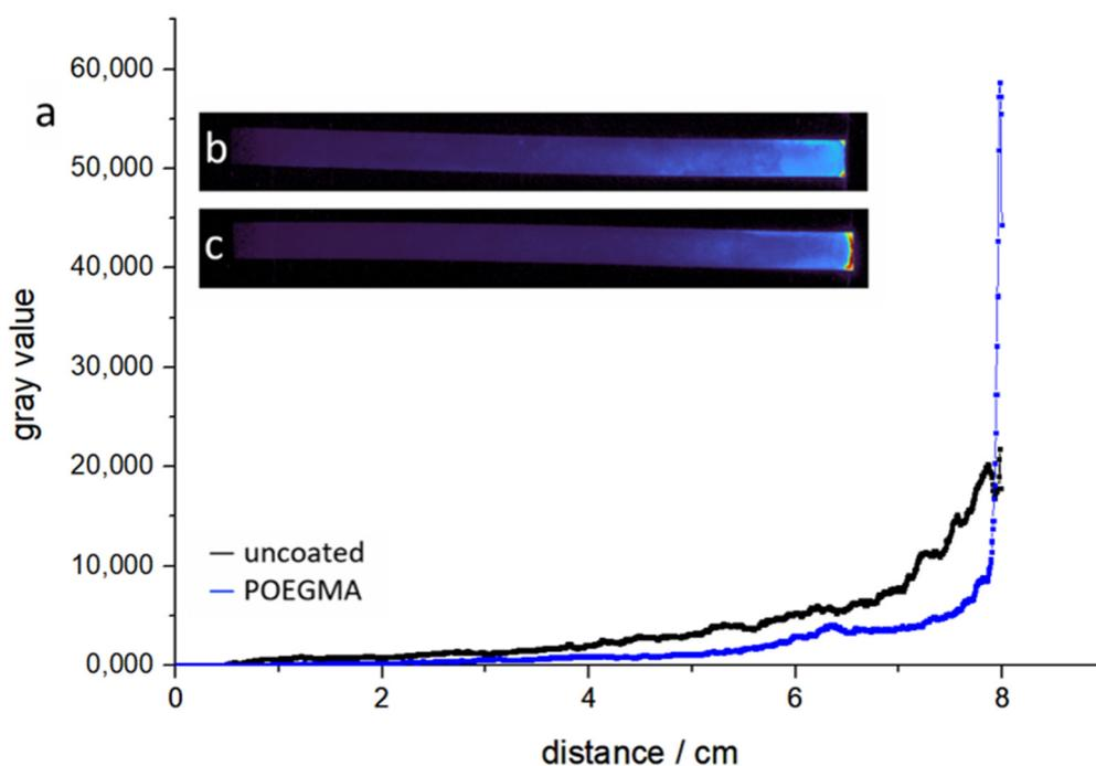
**Figure 10.** A comparison of uncoated and POEGMA-coated paper. In this experiment, BSA-FITC is in a “fully wetted flow” experiment setup. The fluid was evaporated at 7.5–8 cm of the strip for 30 min once the strip was fully soaked. (a) The protein position across the strip by the means of gray values; (b) the fluorescent image of uncoated cotton linters. (c) The fluorescent image of POEGMA-coated cotton linters.
