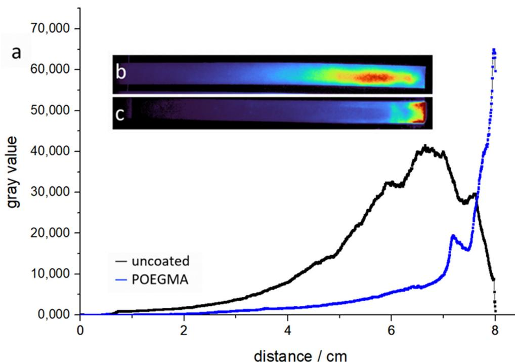
**Figure 11.** A comparison of uncoated and POEGMA-coated paper. In this experiment, GFP with a surface charge of +9 is applied in a “fully wetted flow” setup. The fluid was evaporated at 7.5–8 cm of the strip for 30 min once the strip was fully soaked. (a) The protein position across the strip by the means of gray values; (b) the fluorescent image of uncoated cotton linters. (c) The fluorescent image of POEGMA-coated cotton linters.
