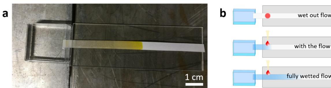
**Figure 6.** (a) Flow experiment with BSA-FITC as the analyte. The paper strip is placed on a PMMA backing and dipped into a fluid reserve, which starts the imbibition process. (b) Representation of the three types of protein application. The top image shows the “wet out flow”, the middle image the “with the flow” or “front”, and the bottom image the “fully wetted flow” setup.
