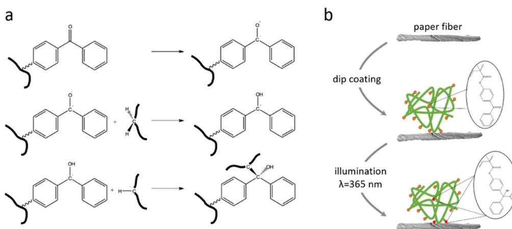
**Figure 1.** (a) Chemical mechanism underlying the crosslinking process. The excited MABP performs a C–H insertion with another molecule via a temporary triplet state. (b) Binding of a polymer chain to a cellulose fiber (not to scale), with the orange dots symbolizing unreacted MABP units and the red dots crosslinked MABP.
