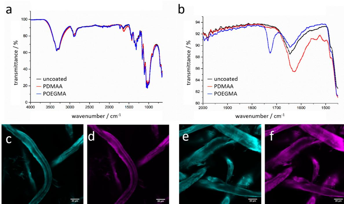
**Figure 2.** IR spectra of uncoated cotton linter paper (black) in comparison with PDMAA-coated paper (red) and POEGMA-coated paper (blue) are shown (a). In a close-up, the changing bands at 1600–1750  $\text{cm}^{-1}$  are clearly visible (b). CLSM images show cotton linter fibers stained with calcofluor white (c,e, cyan), as well as the distribution of PDMAA (d) and POEGMA (f) on the respective fibers (magenta).
