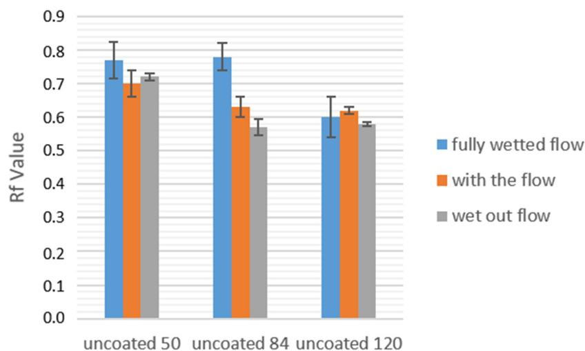
**Figure 7.** A comparison between cotton linter paper strips of different grammage in terms of the resulting  $R_f$  values. The applied protein was BSA.
