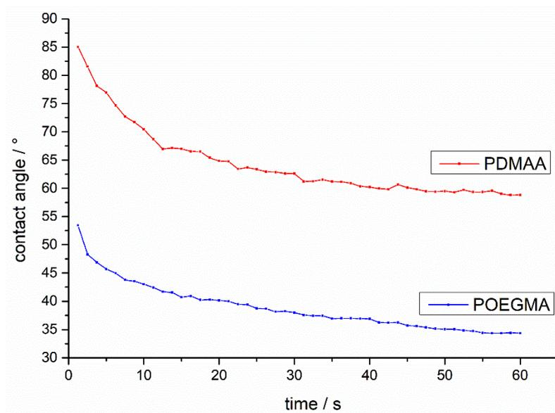
**Figure 4.** Dynamic contact angle measurements of P(OEGMA-co-MABP) and P(DMAA-co-MABP) on a PMMA slide. The coating was applied via dip-coating, crosslinked, and subsequently extracted for 20 min in water.
