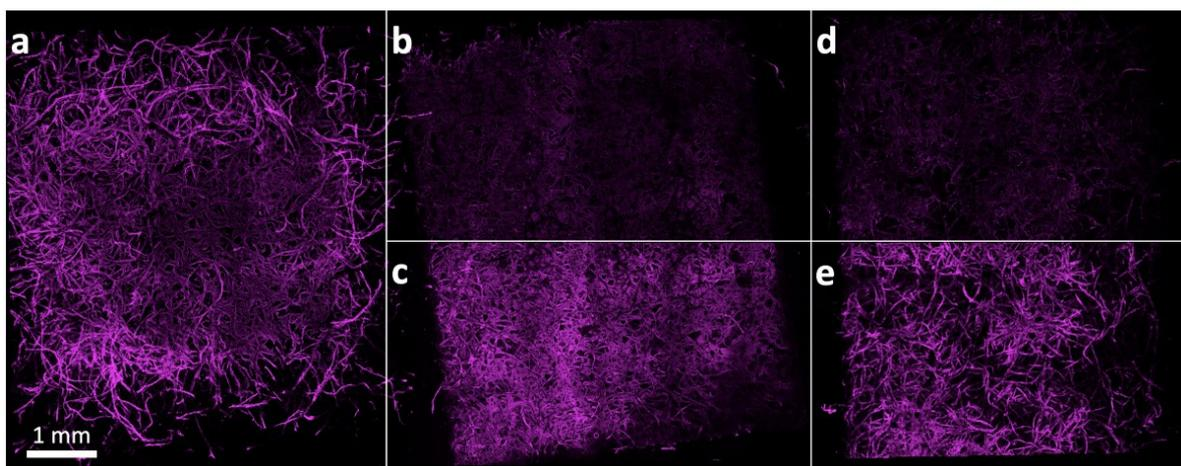
**Figure 5.** CLSM image of three differently treated cotton linter papers, stained with CBM3a-mRuby3: uncoated (a), coated with POEGMA (b,c), and coated with PDMAA (d,e). The bottom half of the POEGMA (c) and PDMAA (e) coated papers is enhanced in brightness for better visualization, while the top half shows the observed intensity in comparison to the uncoated paper.
