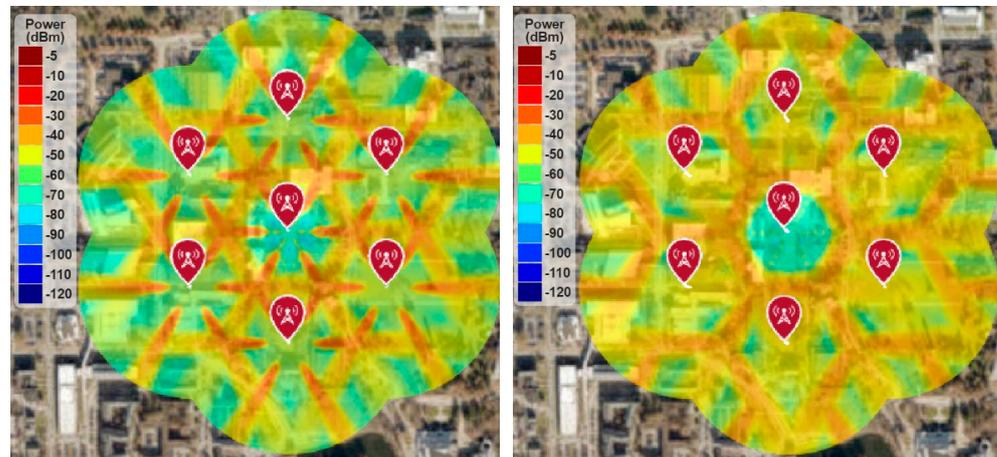
Figure 25. RF coverage and signal strength versus antenna height.
