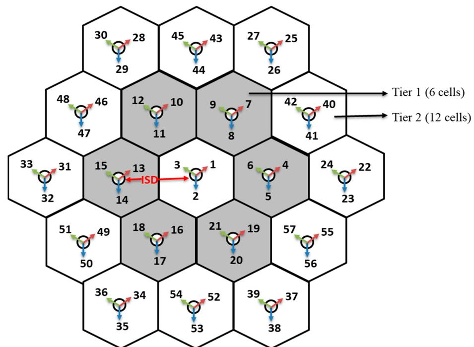
**Figure 4.** 5G Network layout that has 19 cells, each with three sectors.
