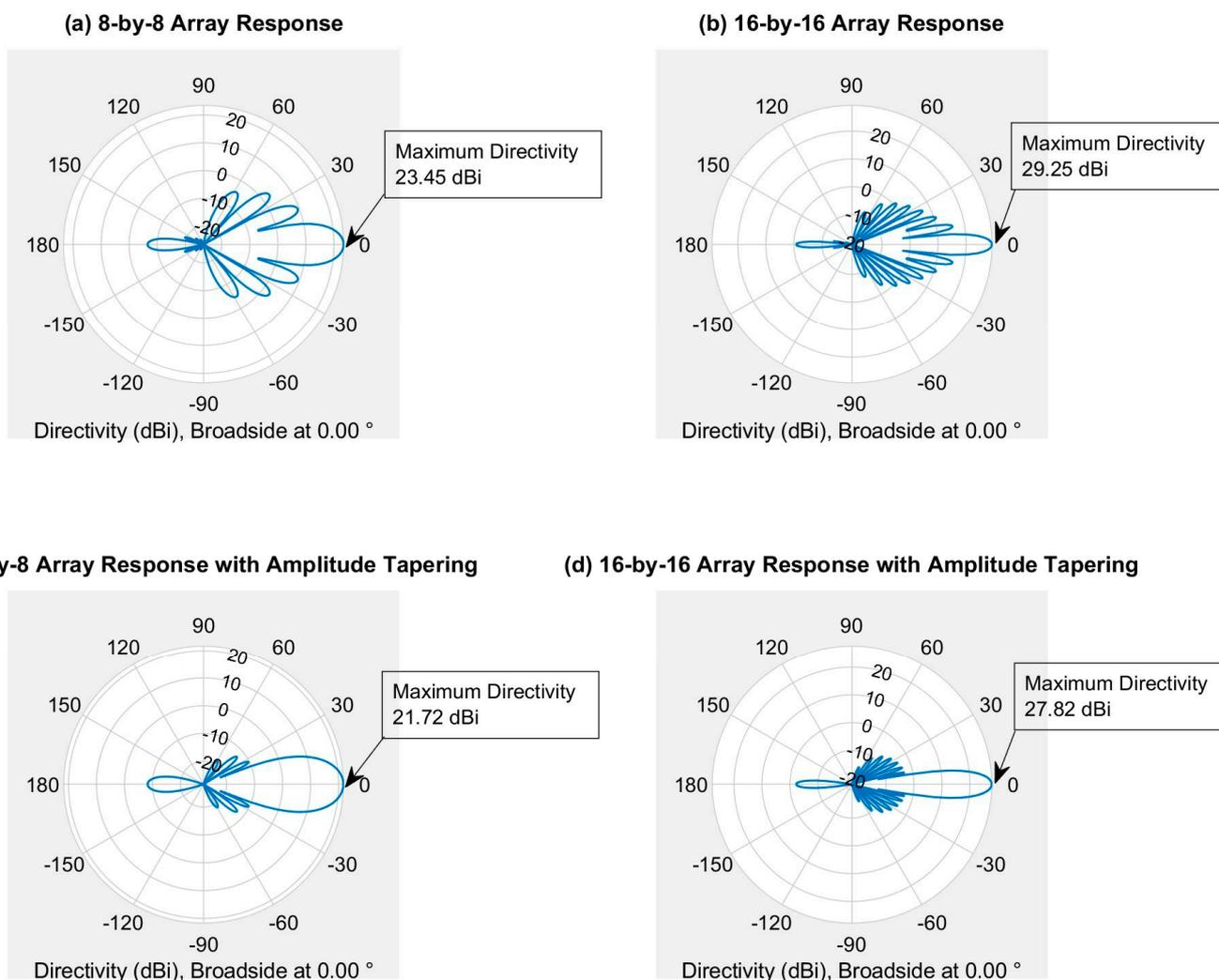
Figure 11. 2D radiation pattern of the array (i.e., 8-by-8 and 16-by-16 array) with and without amplitude tapering.
