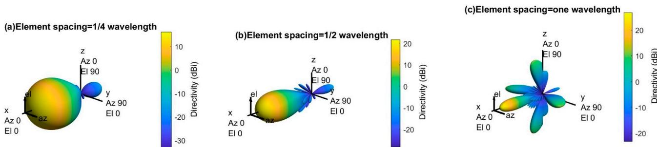
Figure 12. 3D radiation pattern of an 8-by-8 antenna array with different element spacing and reduced sidelobe power.
