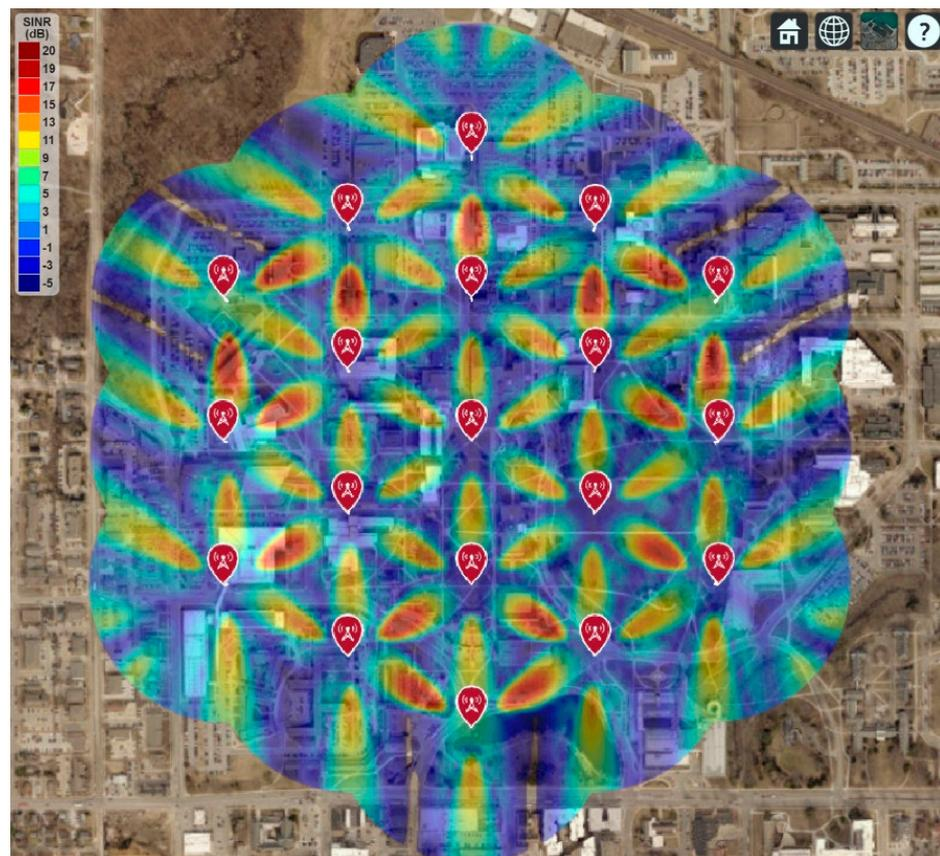
Figure 17. 5G Network Coverage and SINR Map for 8-by-8 Antenna Array.
