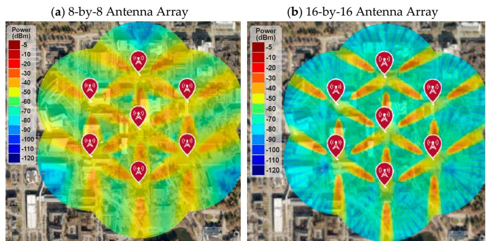
**Figure 19.** RF coverage and signal strength for 30GHz operating frequency.
