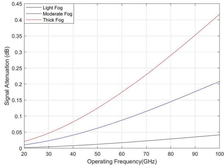
**Figure 15.** RF signal attenuation due to fog for different operating frequency.
