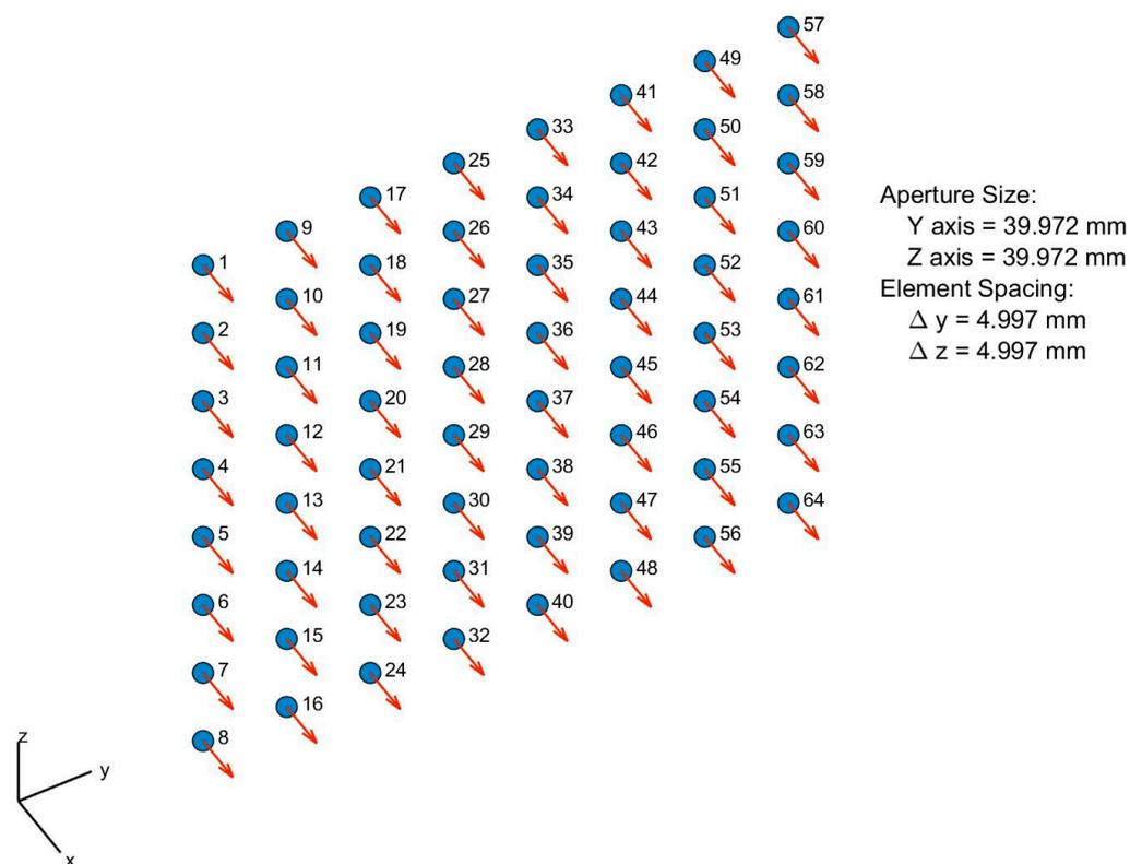
Figure 5. An 8-by-8 uniform rectangular array.
