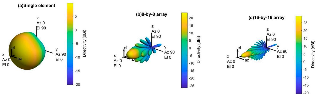
**Figure 8.** 3D radiation pattern of a single site with different array size.
