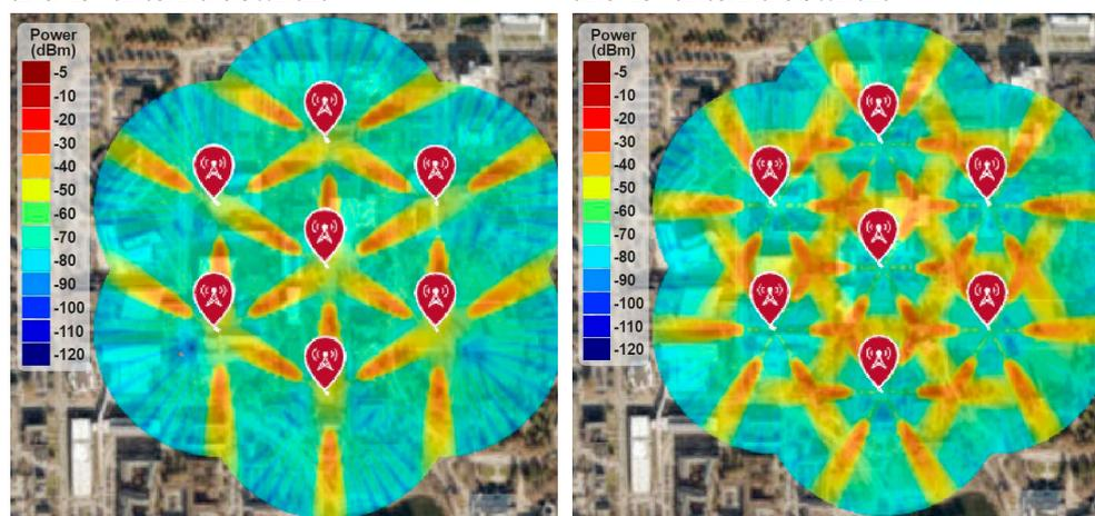
Figure 21. RF coverage and signal strength versus higher-order sectorization.
