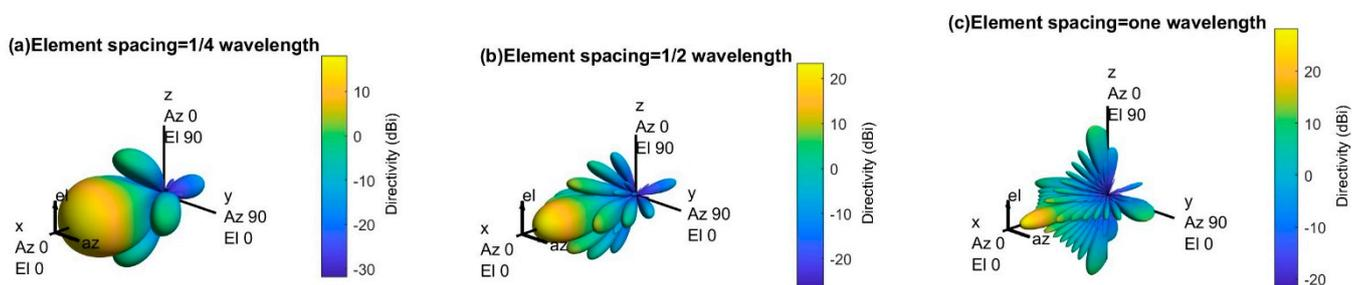
**Figure 7.** 3D radiation pattern of an 8-by-8 antenna array with different element spacing for 30 GHz operating frequency.
