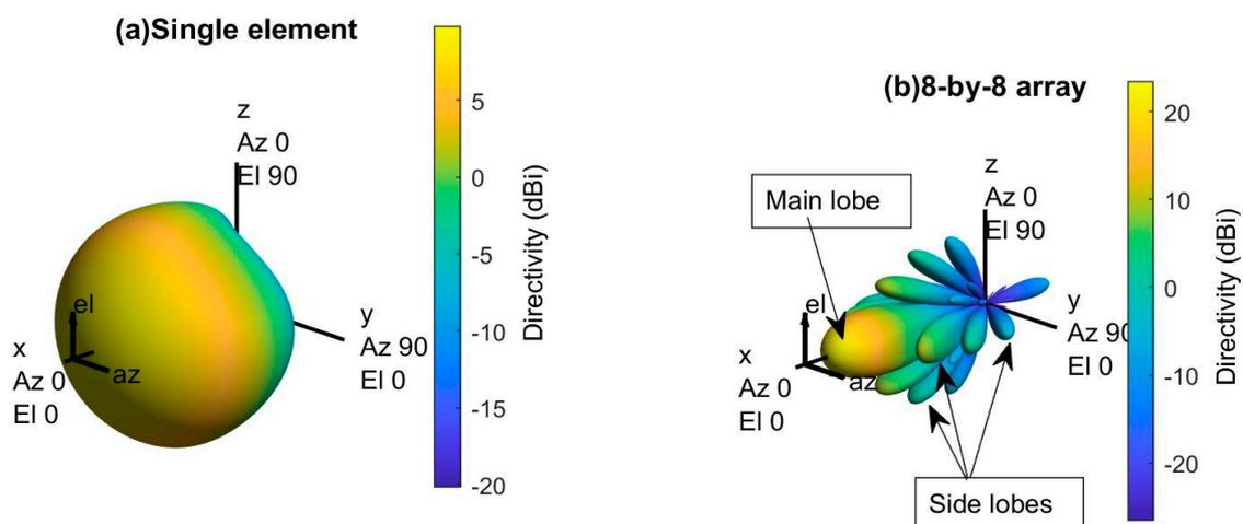
Figure 6. 3D radiation pattern of a single element and an 8-by-8 antenna array for 30 GHz operating frequency.
