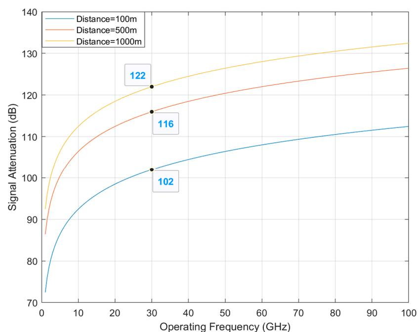
Figure 13. Free space propagation loss for different operating frequency.
