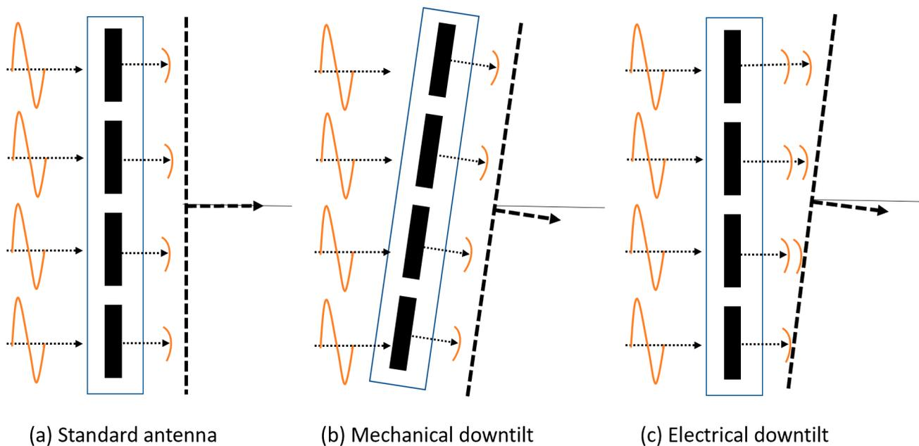
Figure 23. Types of antenna downtilt.
