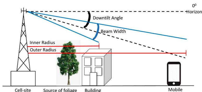
Figure 22. RF coverage with antenna downtilt.
