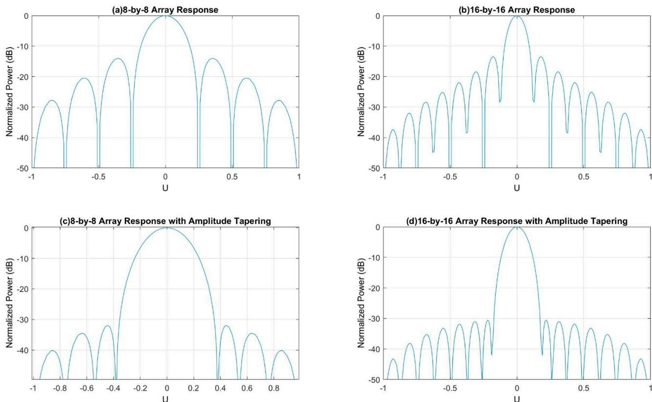
Figure 10. Normalized power distribution of the array (i.e., 8-by-8 and 16-by-16 array) with and without amplitude tapering.
