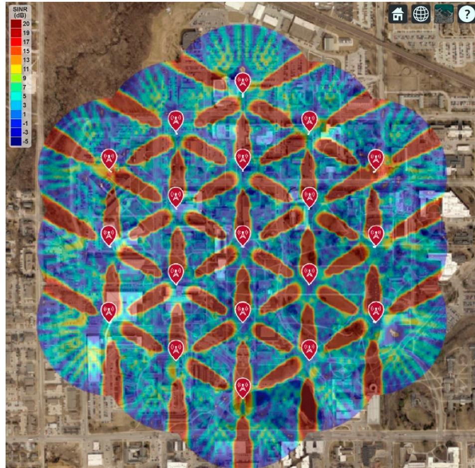
**Figure 18.** 5G Network Coverage and SINR Map for 16-by-16 Antenna Array.
