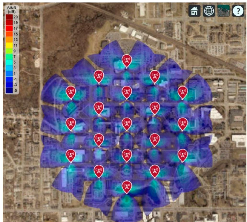
Figure 16. 5G Network Coverage and SINR Map for a single antenna element.
