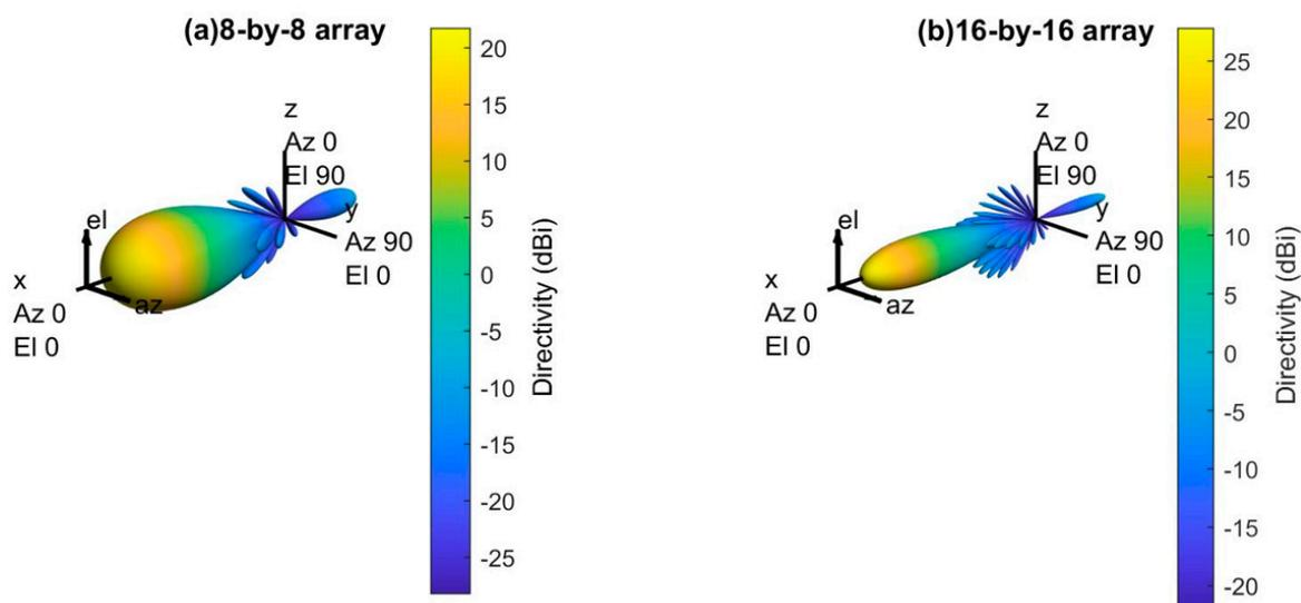
Figure 9. 3D radiation pattern of the array with amplitude tapering.
