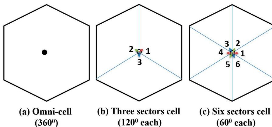
Figure 20. Cell sectorization with directional antennas.
