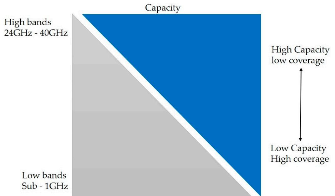
**Figure 2.** Coverage and capacity characteristics of 5G radio frequency ranges.
