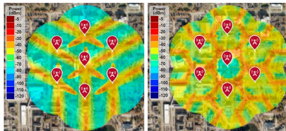
Figure 24. RF coverage and signal strength versus antenna downtilt angle.
