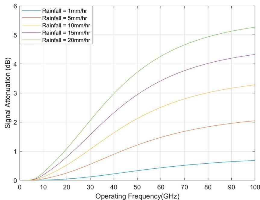
**Figure 14.** RF signal attenuation due to rainfall for different operating frequency.
