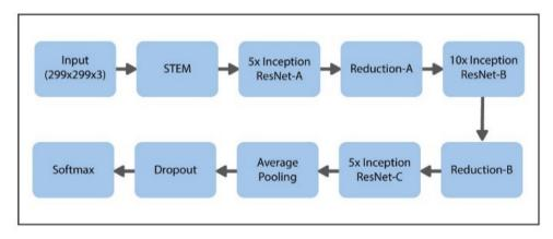
Figure 8. Proposed schema for hybrid Inception-ResNet framework.
