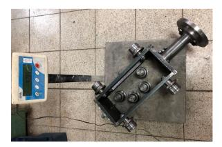
Figure 3. The runner element with attached footpad model.
