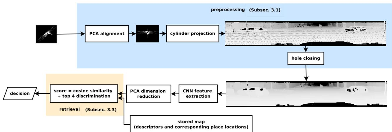
Figure 29. The system overview [82] for point-cloud-based place recognition using CNN feature extraction.
