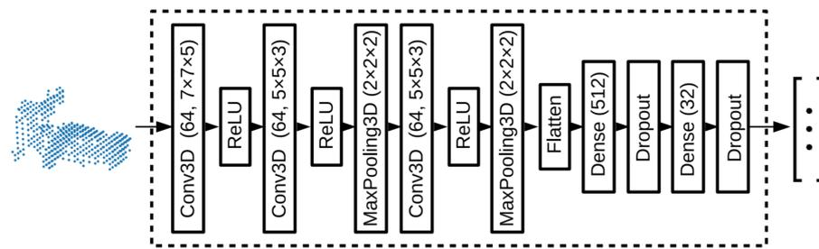
Figure 34. The descriptor extraction network [86] used in the three CNNs.
