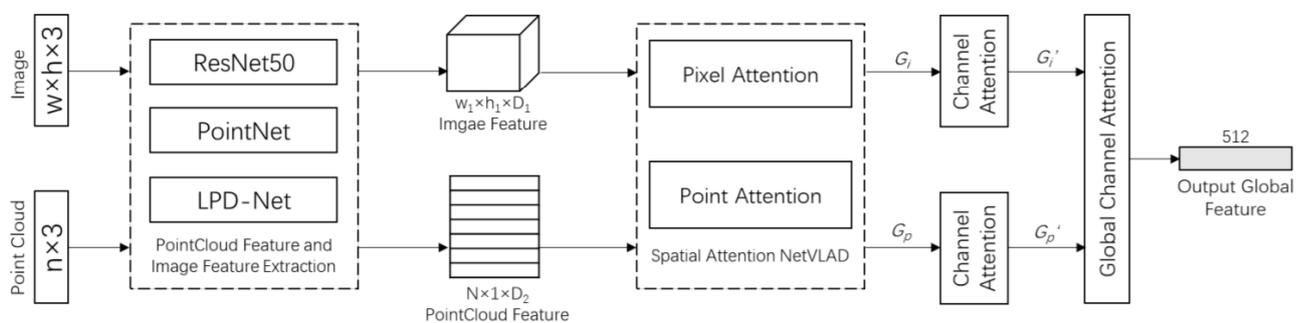
**Figure 37.** PIC-Net [89] composed of image and point cloud branch with spatial, channel, and global attention for large-scale place recognition.
