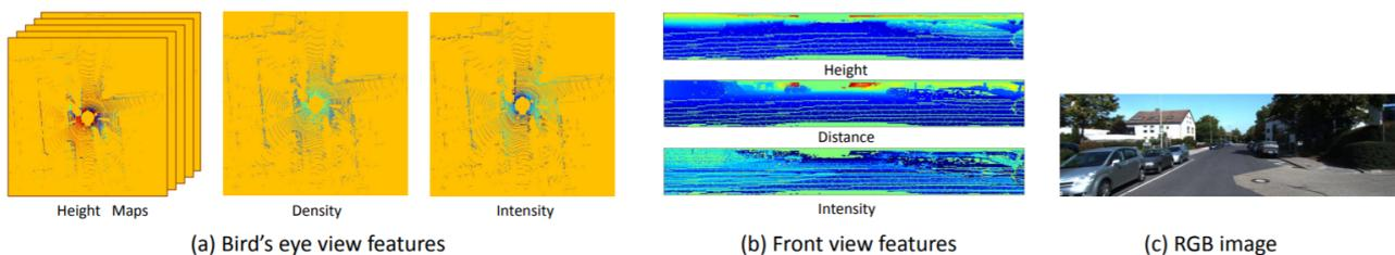
Figure 20. The input features of the MV3D [73] network.
