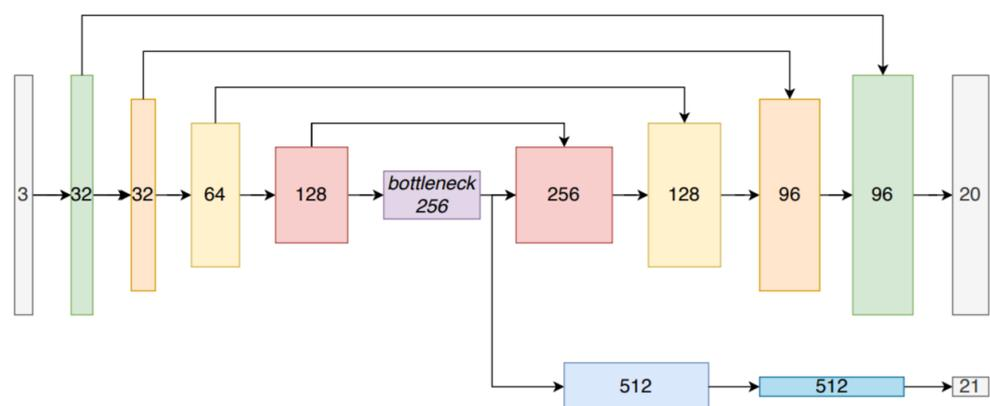
Figure 28. The multi-task network structure [81] for scene recognition in indoor environments.
