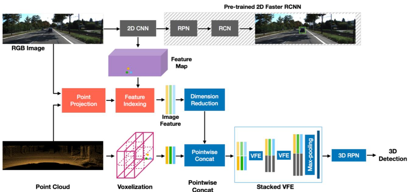
Figure 23. The overview of the MVX-Net [76] PointFusion method.
