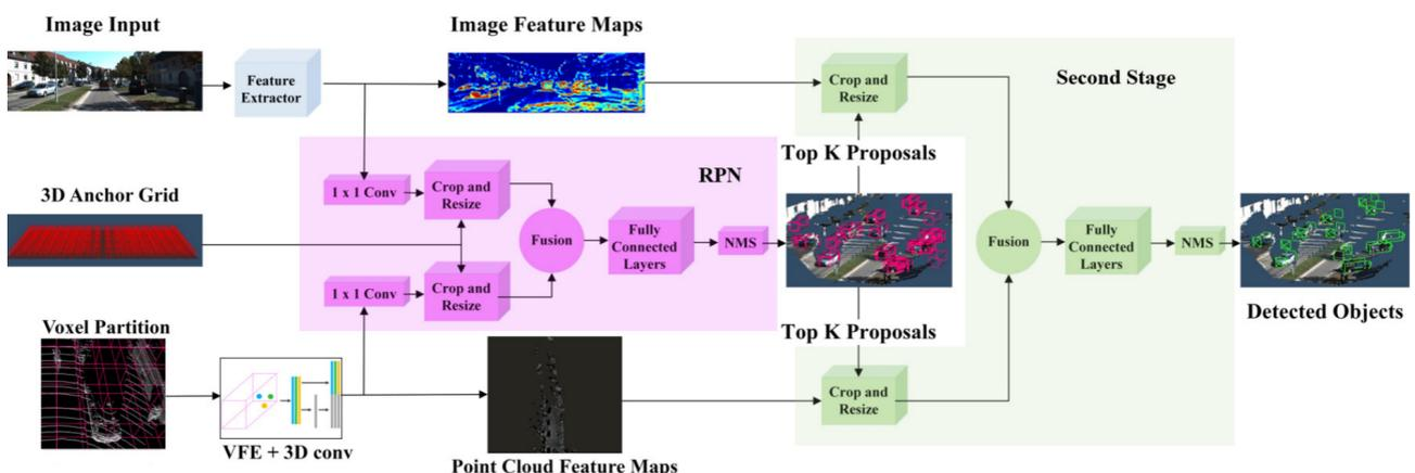
**Figure 22.** Aggregate view object detection [120] network pipeline for 3D object detection in the context of autonomous driving.
