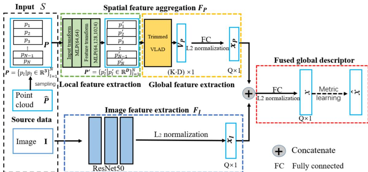
Figure 36. CNN based Camera-LiDAR Fused descriptor [88] for place recognition.
