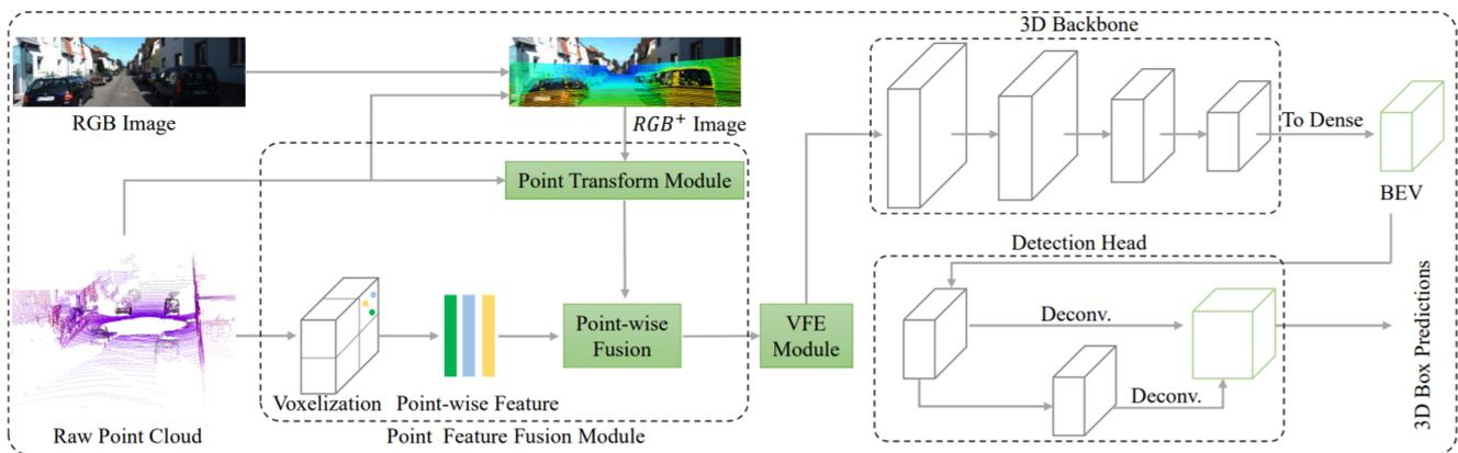
**Figure 24.** The pipeline of 3D object detection [77] network for the LiDAR and camera, including input, the point feature fusion module, the 3D backbone, and the detection head.
