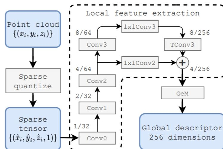
Figure 35. The network of MinkLoc3D [87] for point-cloud-based place recognition.
