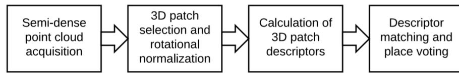
Figure 32. The pipeline of [85] place recognition pipeline in semi-dense maps.
