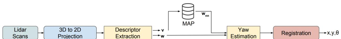
Figure 31. The methodology [84] of oriented recognition from 3D point clouds.
