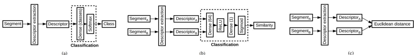
Figure 33. Three network structures [86] (a) group based CNN (b) Siamese CNN, and (c) descriptor extraction CNN trained using contrastive loss.
