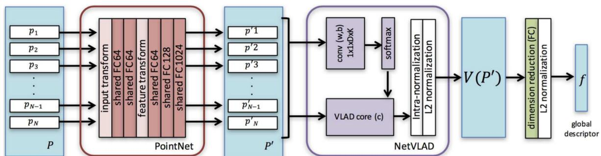
Figure 27. The architecture of our PointNetVLAD [80] network.
