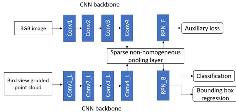
**Figure 21.** The fusion-based one-stage object detection [74] network.
