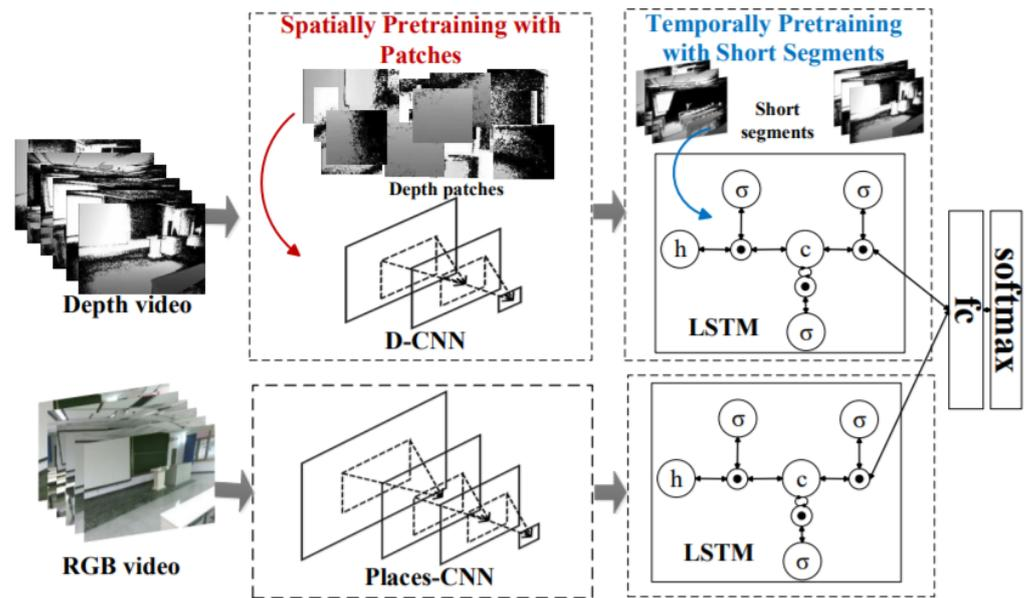
Figure 25. The CNN-RNN [78] architecture for video recognition.
