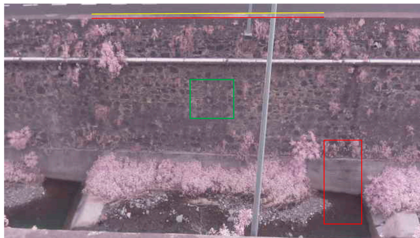
Figure 2. Image taken by the camera with the used control points (lines and green rectangle) and the ROI (red rectangle).
