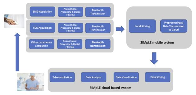
**Figure 2.** The SIMpLE system general architecture which consists of a data acquisition module (commercial sensors), a mobile system and a cloud-based system.
