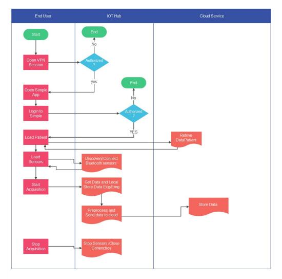
Figure 5. Flow chart relative to the communication between SIMpLE modules.
