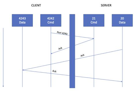
Figure 3. TCP/IP commands scheme.
