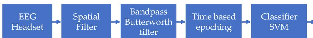
**Figure 5.** Data flow of SVEEP signal.
