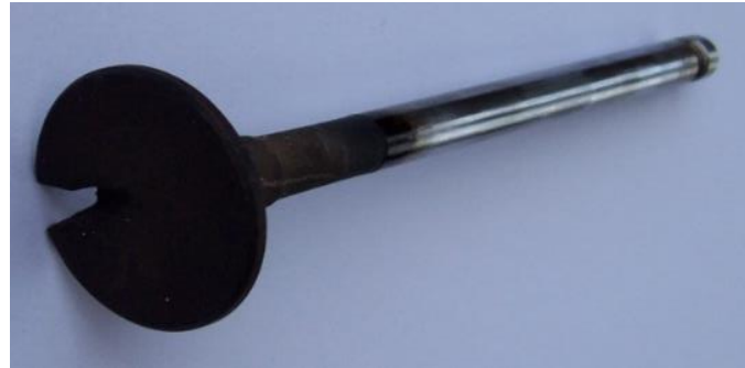
Figure 13. View of the damage of outlet valve.
