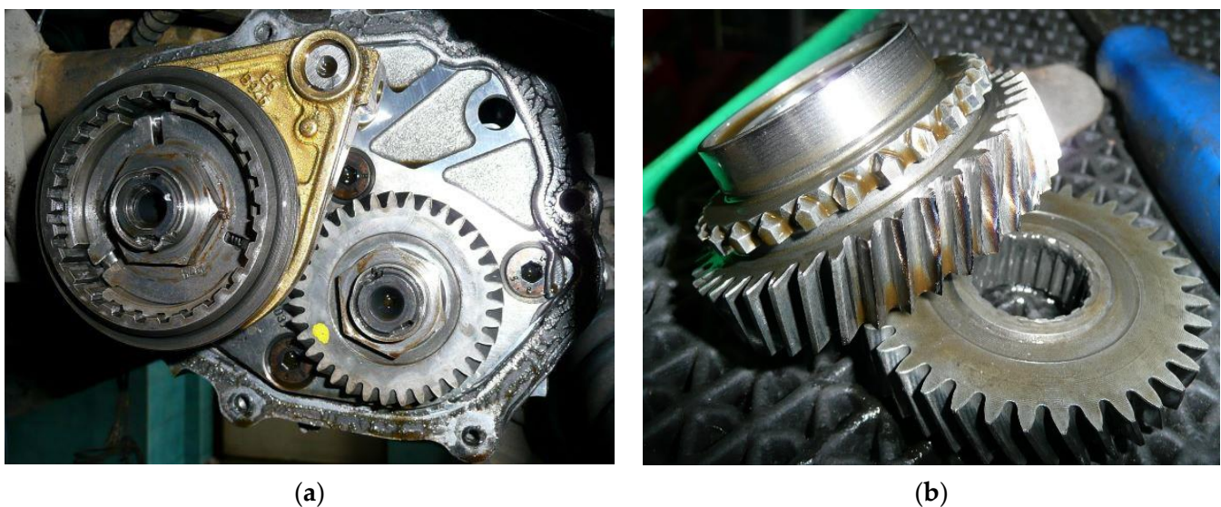
Figure 9. Test object (a) view of the gearbox, (b) pair of gear wheels with signs of wear.
