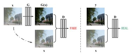
**Figure 1.** The architecture of the proposed framework. "G" denotes the generator and "D" denotes the discriminator. "x" is the input hazy image, "G(x)" is the reconstructed hazy-free image and "y" is the clear image. Unlike the unconditional GAN framework, both the generator and discriminator observe the input hazy image.
