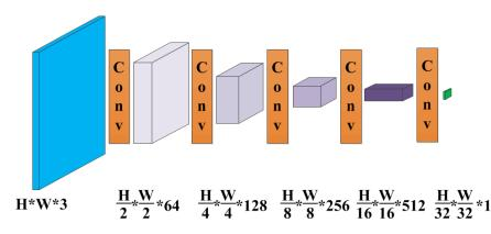
**Figure 7.** The PatchGAN architecture as the discriminator. Each "Conv" contains sequence Conv-BN-ReLU. The kernel size of each convolution operation is  $3 \times 3$ , the stride is  $2 \times 2$ , and the padding is  $1 \times 1$ . The input and output channel numbers can be obtained according to the parameters in the figure.
