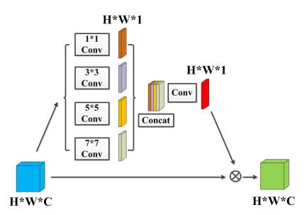
**Figure 6.** SA Block: The spatial attention module. Each "Conv" contains sequence Conv-BN-ReLU, "Concat" refers to concatenation. The kernel size of the last convolution operation is  $3 \times 3$ , the stride is  $1 \times 1$ , and the padding is  $1 \times 1$ . The input and output channel numbers are 4 and 1, respectively.
