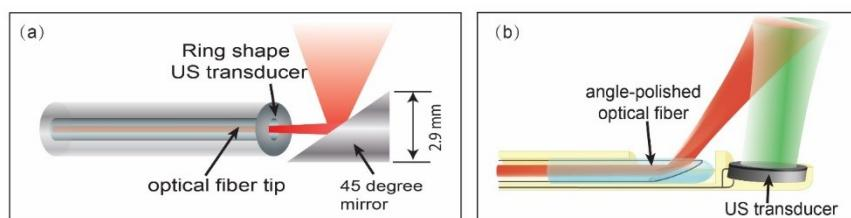
**Figure 5.** Schematic of different IVPA catheter designs. (a) Schematic of a collinear IVPA catheter design. (b) Schematic of an IVPA catheter with a longitudinal offset between optical and acoustic beams (red optical beam and green ultrasound beam). Reprinted from [114] with permission.
