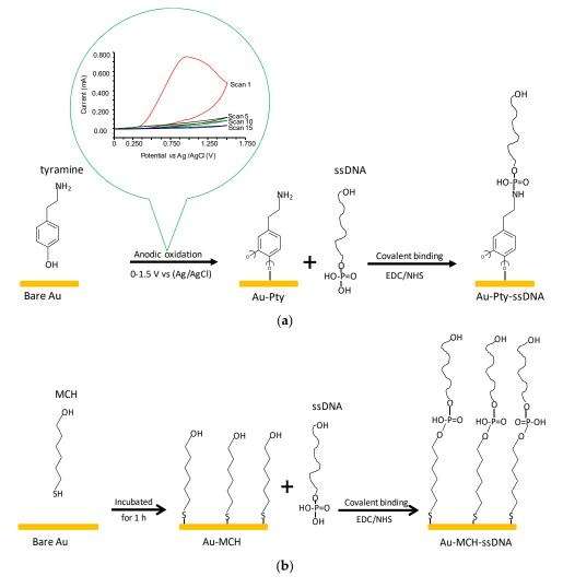
**Figure 1.** (a) Sensor chip surface modified with Pty film and followed by addition of ssDNA to form phosphoramide ester bond. The inset shows the reduction in anodic peak current during electropolymerization of tyramine on the sensor chip surface (scan numbers 1, 5, 10 and 15). (b) Sensor chip surface modified with MCH-SAM and followed by addition of ssDNA to form phosphate ester bond.
