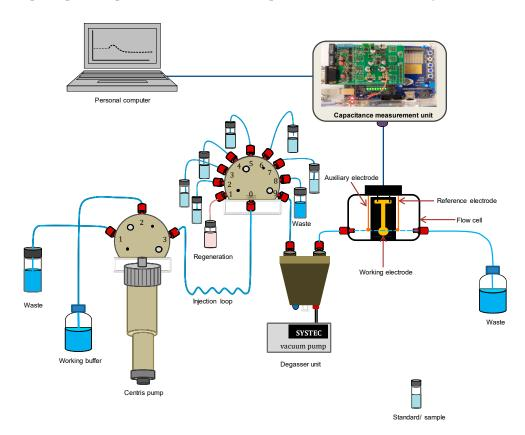
Figure 2. Schematic drawing of the flow-injection analytical system (CapSenze™ Biosystem).
