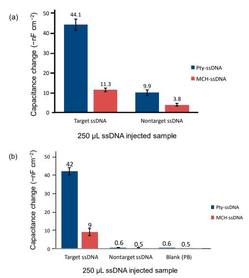
**Figure 7.** The amplitude of responses from Pty-ssDNA and MCH-ssDNA sensor chips to injection of equimolar concentrations,  $10^{-8}$  M, of target and non-target ssDNA samples at (**a**) 23 °C (RT) and (**b**) 50 °C hybridization temperatures, respectively.
