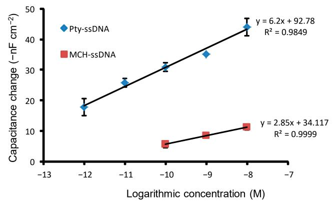
**Figure 6.** Calibration curves showing linearity range for target ssDNA hybridized with capture probe on the different sensor chips modified with Pty-ssDNA and MCH-ssDNA.
