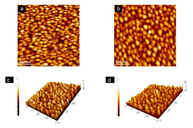
**Figure 5.** Non-contact mode AFM images (scan size  $1 \ \mu m \times 1 \ \mu m$ ) of (**a**) gold sensor chip surface after being modified with Pty and coupled with ssDNA, and (**b**) gold sensor chip surface after being modified with MCH and coupled with ssDNA. The three-dimensional (3D) images of (**a**,**b**) are shown in the figures marked (**c**,**d**), respectively.
