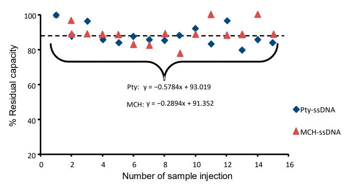
**Figure 8.** Reusability of Pty-ssDNA- and MCH-ssDNA-modified sensor chips. A total of 250  $\mu$ L of a 10<sup>-9</sup> M target ssDNA was applied 15 times on each sensor chip with a regeneration step between each individual assay. Symbols represent averages of triplicate data collected from CapSenze<sup>TM</sup> Biosystem.
