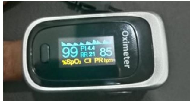
**Figure 11.** Pulse oximeter used for measuring RPM.
