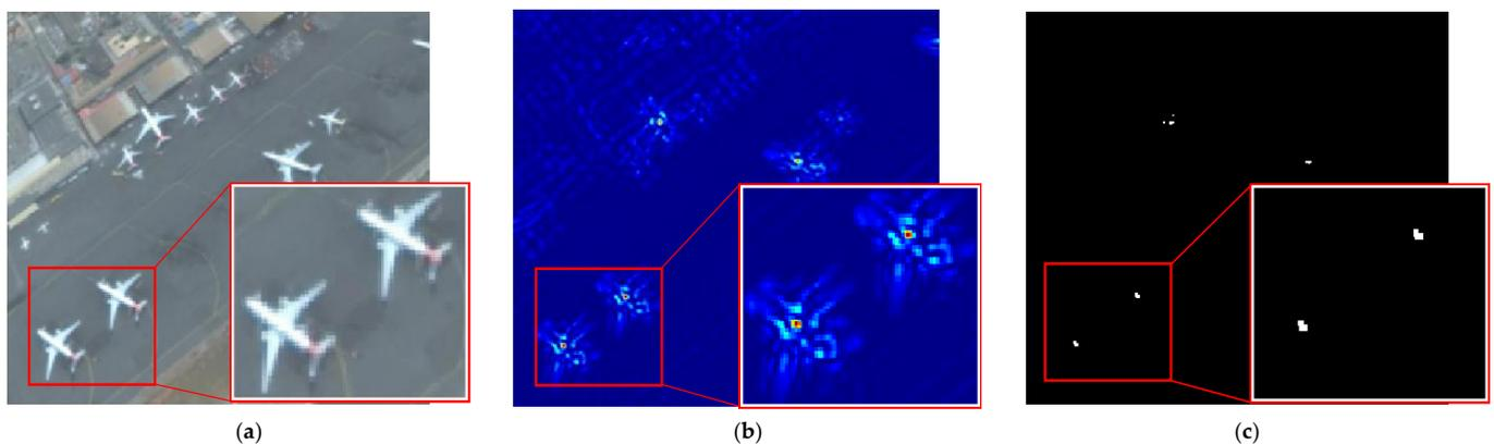
**Figure 5.** The Original RSI and the process of target center determination. (a) The original RSI with the resolution of  $1121 \times 957$  pixels; (b) the corresponding center-response magnitude map generated by a convolution kernel ( $r = 20$  pixels); (c) the binary image with the center of targets obtained by threshold segmentation.
