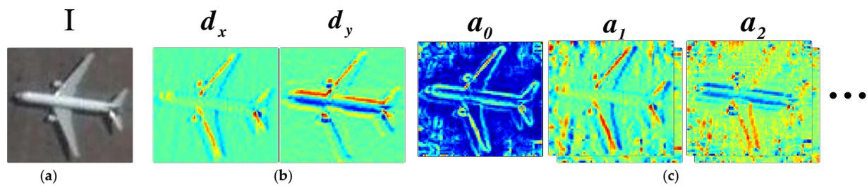
**Figure 7.** Illustration of the expansion of gradient images to Fourier coefficient images. (a) The input image; (b) the gradient image; (c) the complex Fourier coefficient images.
