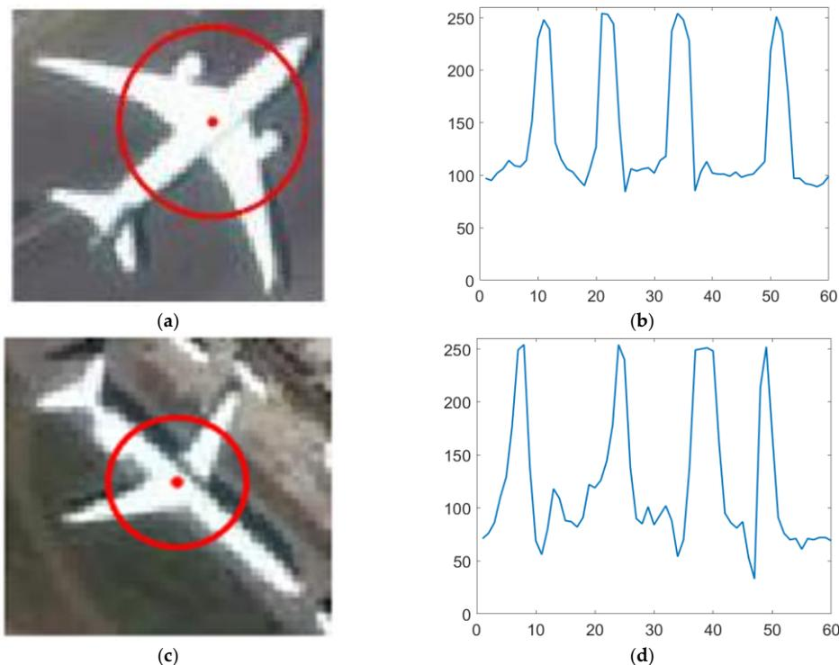
**Figure 3.** The aircraft and corresponding circular intensity signal waveform charts. (a,c) Aircraft in RSIs; (b,d) circular intensity signal waveform charts centered at aircraft's central point.
