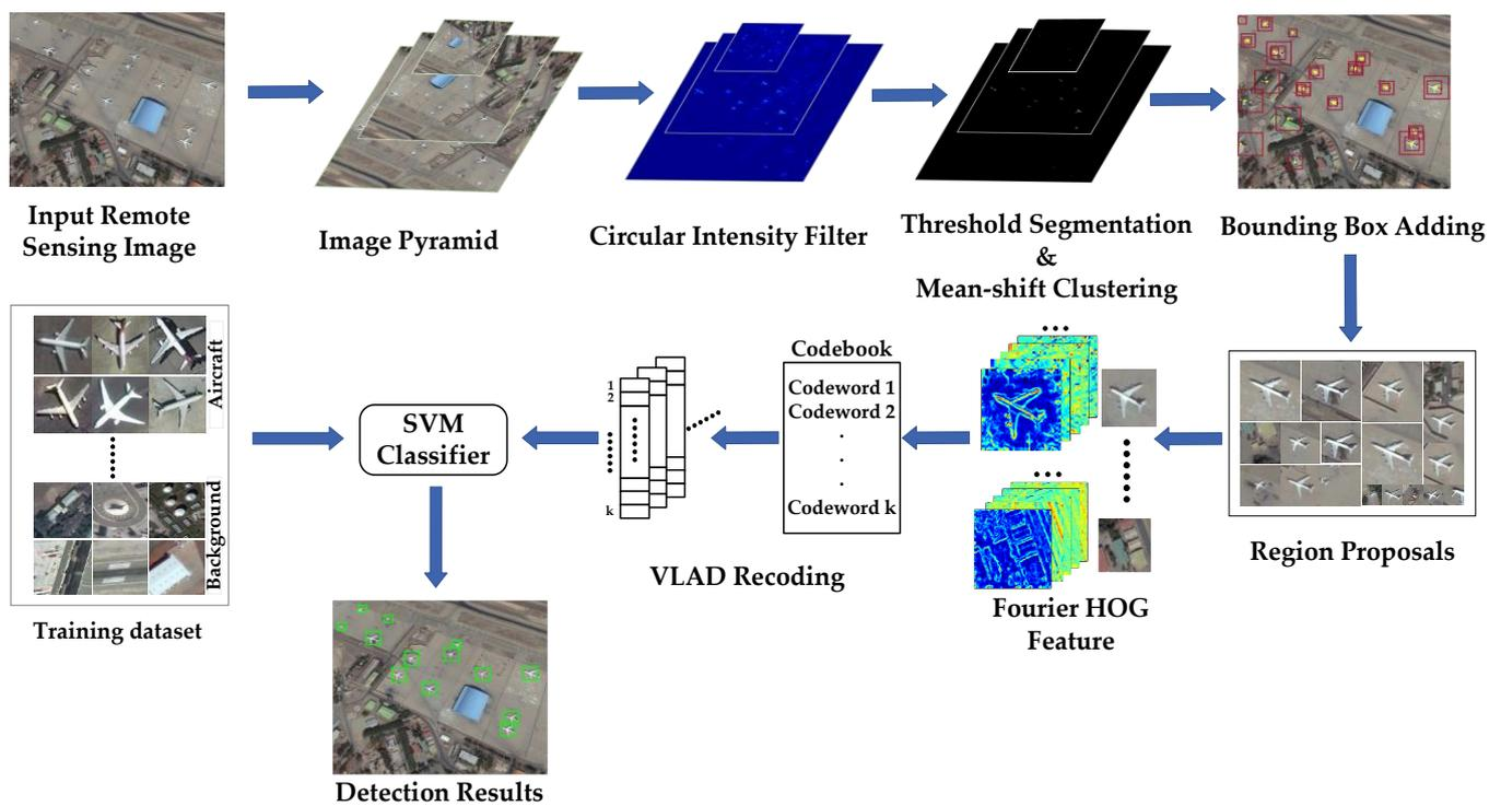
Figure 2. The flowchart of the proposed aircraft detection scheme.
