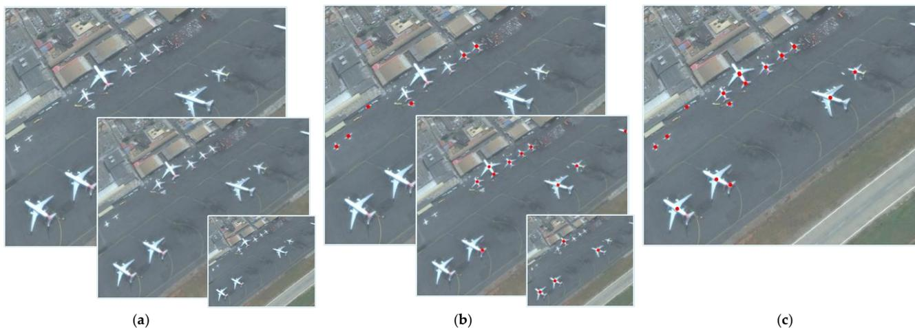
**Figure 6.** Multi-scale image pyramid and the results of aircraft target center determination. (a) RS image pyramid; (b) center determination on image pyramid; (c) center point aggregation.
