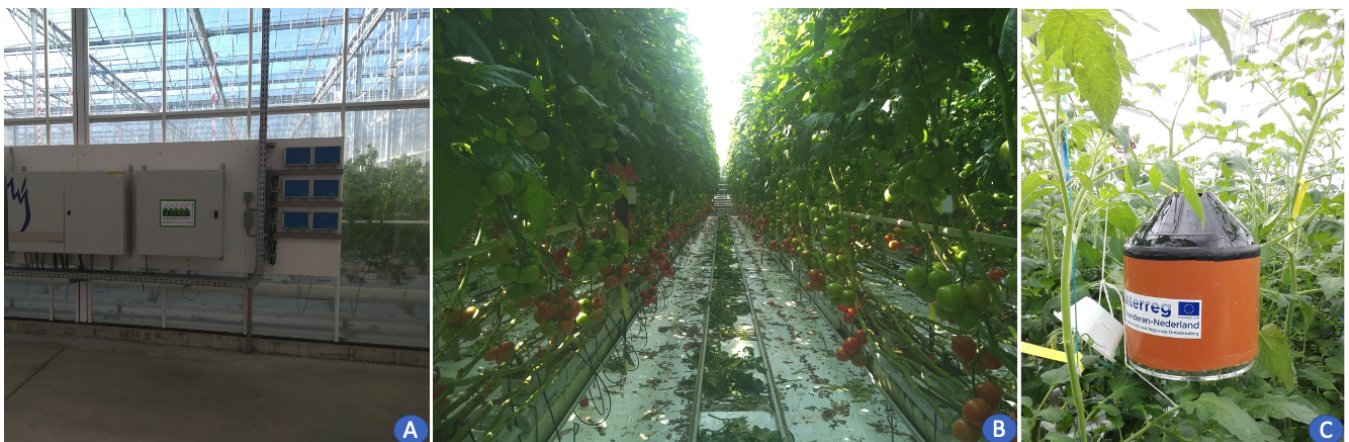
Figure 5. Greenhouse layout and sensor deployment in the greenhouse. (A) Complex infrastructure of the greenhouse. (B) Row of plants inside the greenhouse. (C) Sensor deployment in the greenhouse (air-flow (AF) boxes).
