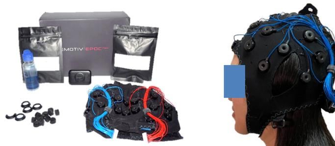
Figure 1. EPOC Flex 32-channel wireless EEG device.
