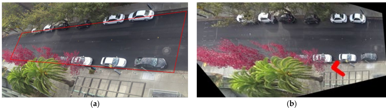
Figure 9. Comparison before and after image preprocessing. (a) is the picture before processing, (b) is the result of highlighting the target pedestrian and perspective transformation.
