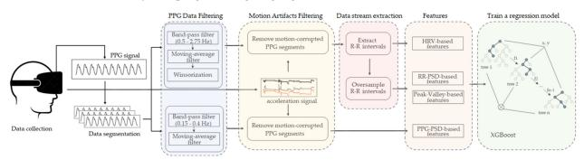
**Figure 6.** Block diagram of the proposed ML-based method for breathing rate estimation from PPG data acquired from a head-mounted device (VR headset).
