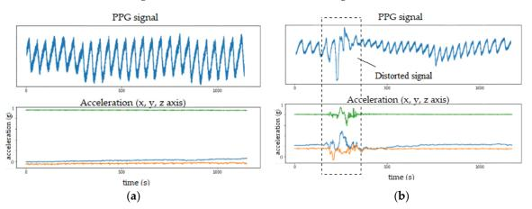
**Figure 7.** Illustration of the effect of motion on PPG signals: (**a**) clean PPG waveform when no motion is present; (**b**) PPG signal affected by motion artifacts during movement.
