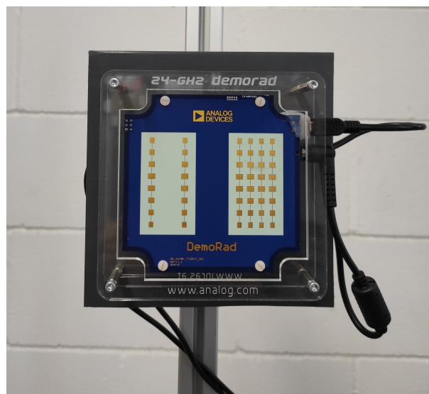
Figure 16. Image of EVAL-DEMORAD kit used in the experiments.
