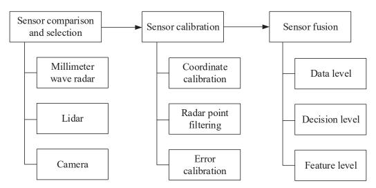
Figure 1. Process of mmWave radar and vision fusion.
