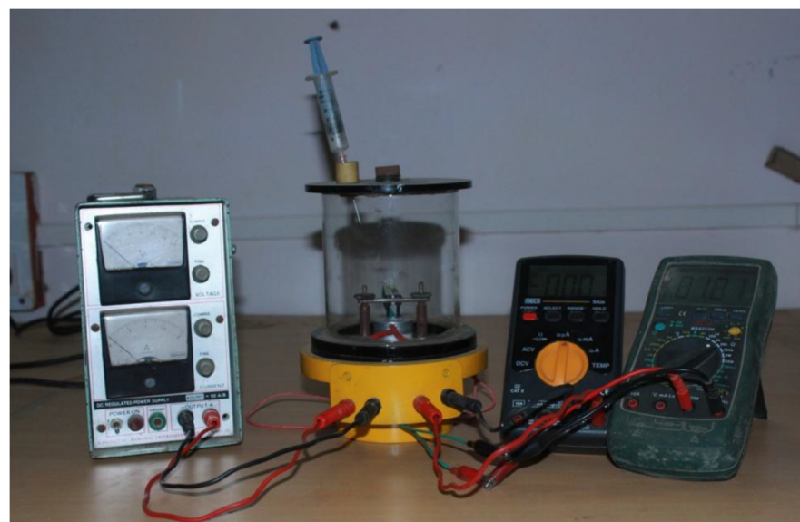
Figure 5. (a) Schematic diagram of proposed gas-sensor unit. Reprinted from [68] under CC BY-NC licence; (b) Photograph of the proposed gas-sensor set-up. Reprinted from [68] under CC BY-NC licence.
