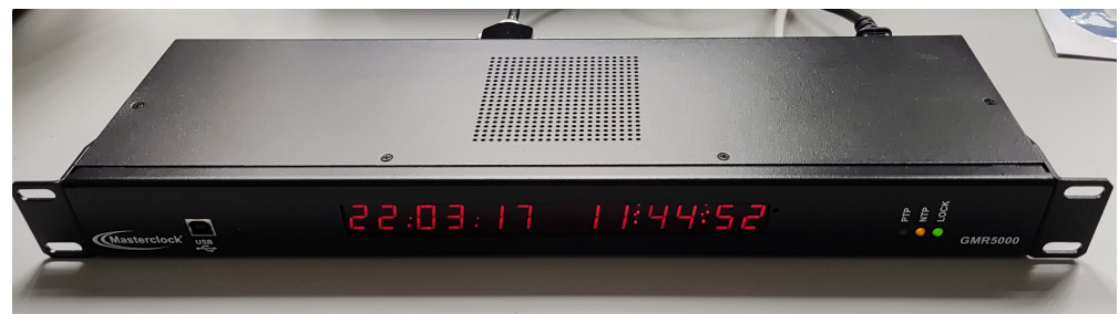
Figure 6. GMR5000 (from Masterclock Inc., St Charles, MO, USA) as an NTP local server used for time syncing.
