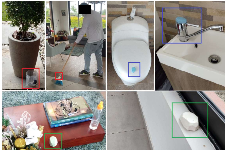
Figure 3. Beacons deployed. The two mobile beacons are in red squares (in jug and broom). Two of the six active beacons are in blue squares (toilet and bathroom sink). Two of five stationary beacons in green squares (living room and corridor).
