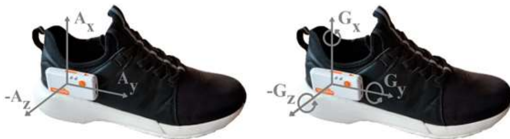
Figure 2. Axis alignment of the IMU attached to the right shoe of each participant.
