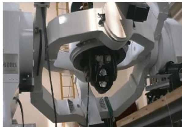
Figure 18. Swing table experiment of aviation photoelectric stabilization platform.
