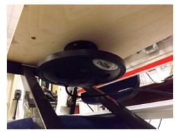
**Figure 9.** Experimental setup for studying vibrotactile feedback on digital piano (**right**). One of the transducers used to convey vibration at the keyboard (**left**).
