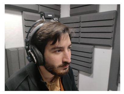
**Figure 10.** Motion-tracking headphones. By controlling the individual HRTF structural model, it allows perceiving the position of the virtual sound source independent of head movements.
