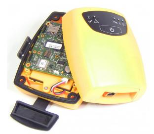
**Figure 18.** X-Poles is fixed to the pole through an elastic strap. The test starts with a vibration measurement generated by a hammer. Using a built-in accelerometer, the device collects the pole vibrations and then extracts the natural eigenfrequency and evaluates the Ultimate Breaking Strength of the pole.
