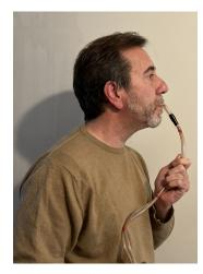
**Figure 5.** The interface designed for detecting postures of the oral cavity. It has a small loudspeaker, a microphone and two physical waveguides: one feeds white noise inside the mouth, and the other picks up the signal filtered by the oral cavity.
