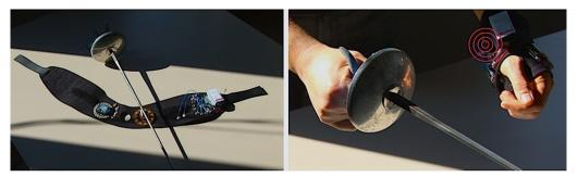
**Figure 17.** Glove with wrist strap for radio communication from the fencer to the scorekeeper and for actuator control.
