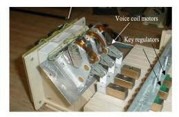
Figure 8. The Multi-Instrument active KEYboard (MIKEY) with a force feedback to the touch.
