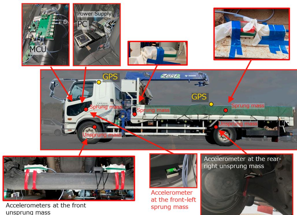
Figure 1. Vehicle and Accelerometers installation point.
