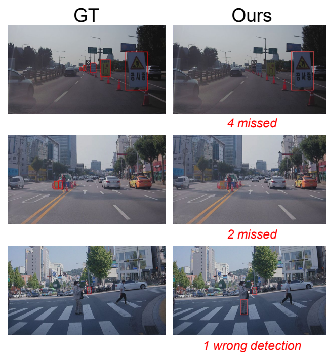
Figure 12. Limitations: if the construction sign is severely occluded, we cannot detect it accurately (first and second rows). A rectangle shape can be detected as a construction sign (third row).
