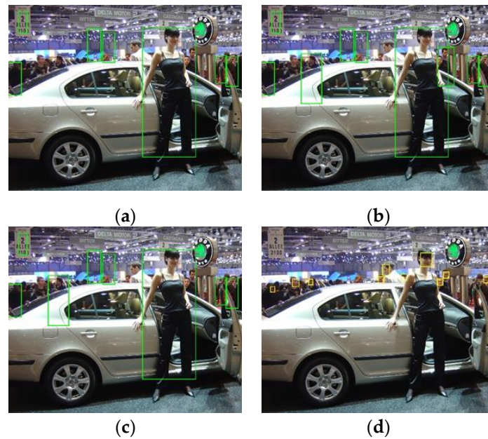
Figure 10. Detection results of the ACF detector (a), the integrated detector with r_w = r_h = 0 (b) or r_w = 3, r_h = 8 (c) and the MTCNN detector (d). In (b), there are 2 more false positives than in (a), while (c) only has one more false positive.
