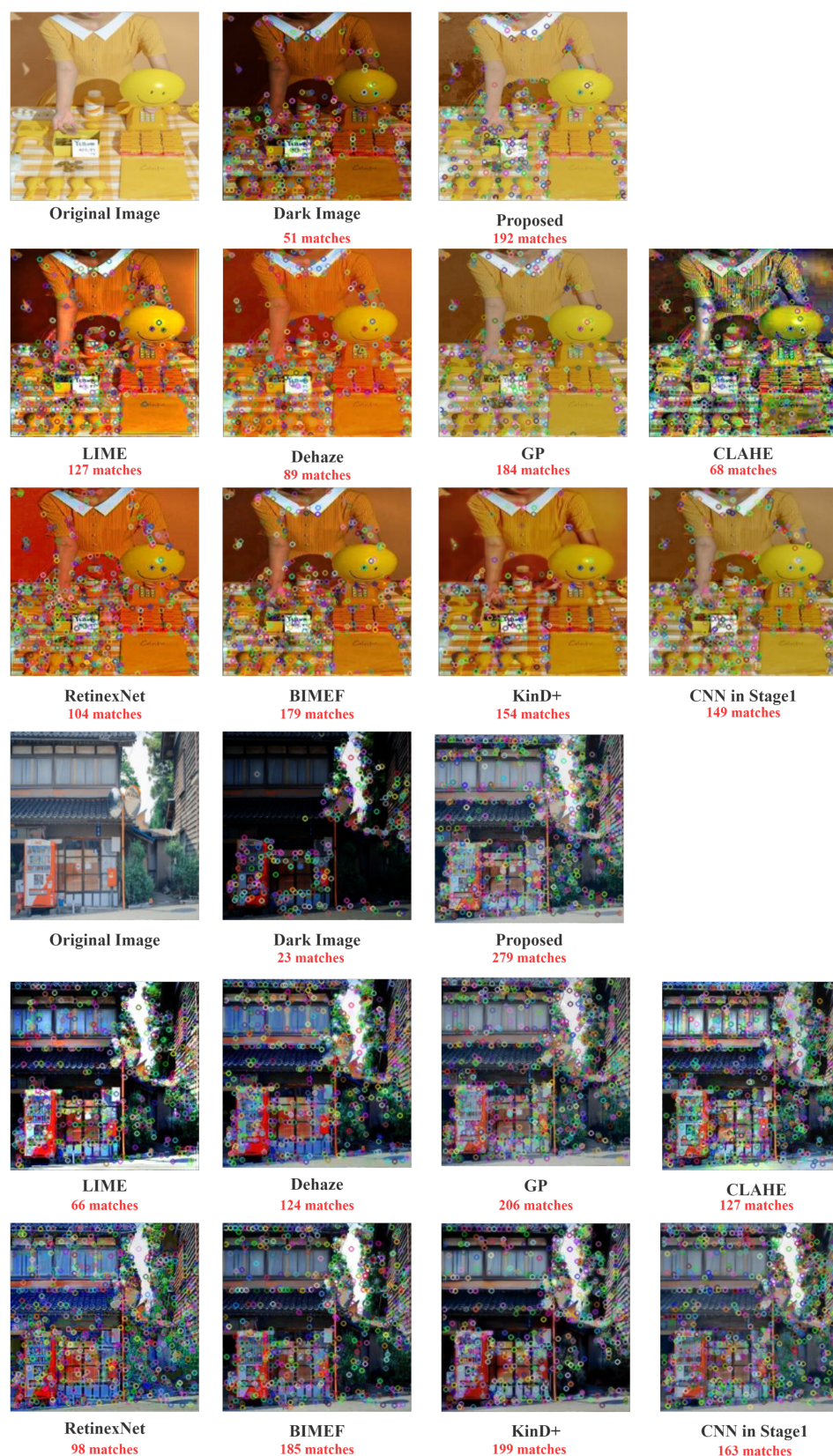
Figure 9. SIFT features matched in synthetic low-light images using different enhancement methods.
