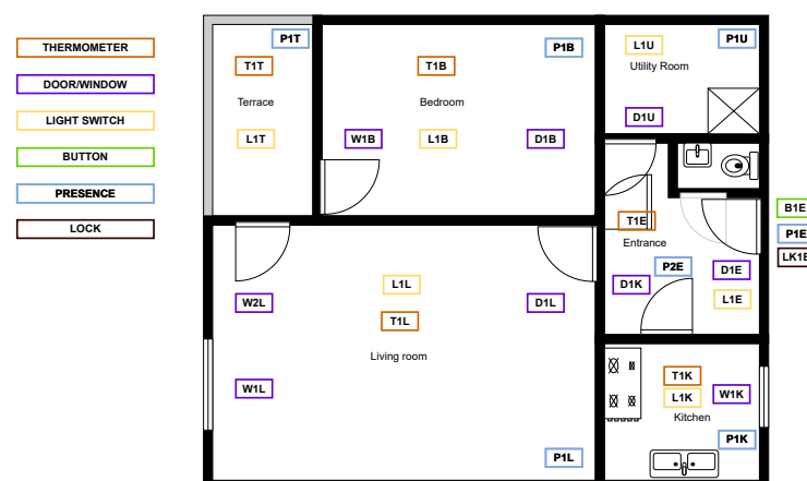
Figure 3. The schema represents the floor-plan of typical domestic environment equipped with various domotic IoT devices.
