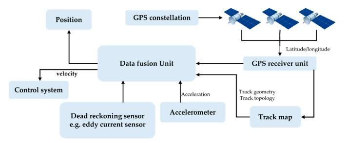
Figure 6. Main components of a railway vehicle positioning.
