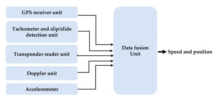
Figure 7. Integration of different sensors for measuring train position and speed.
