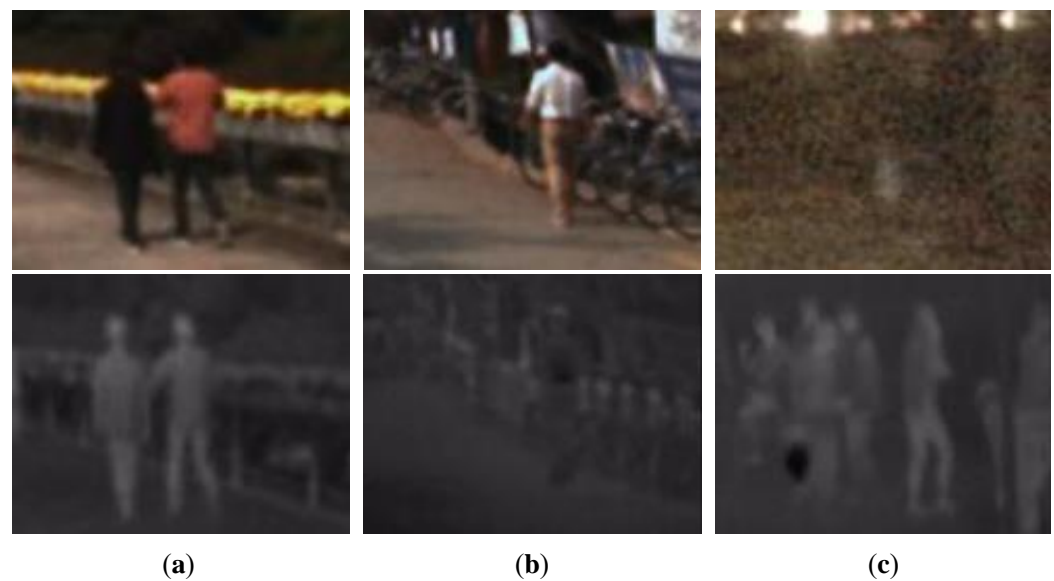
Figure 1. Typical samples of multispectral pedestrian images. The first and second row are visible and thermal images, respectively. (a) Both visible and thermal images are captured in good conditions. (b) Thermal image is captured at ambient temperatures similar to the body temperature and the thermal crossover may occur, leading to blurred and low-contrast results, while the quality of visible image is still good. (c) Visible image is captured under an extreme lighting condition, while their paired thermal image is robust against the illumination change.
