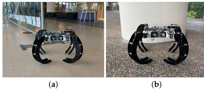
**Figure 9.** Crawling locomotion mode. (a) On smooth surface. (b) On rough surface.
