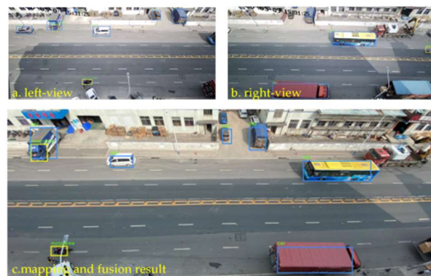
Figure 3. Object detection from different angles based on image fusion.
