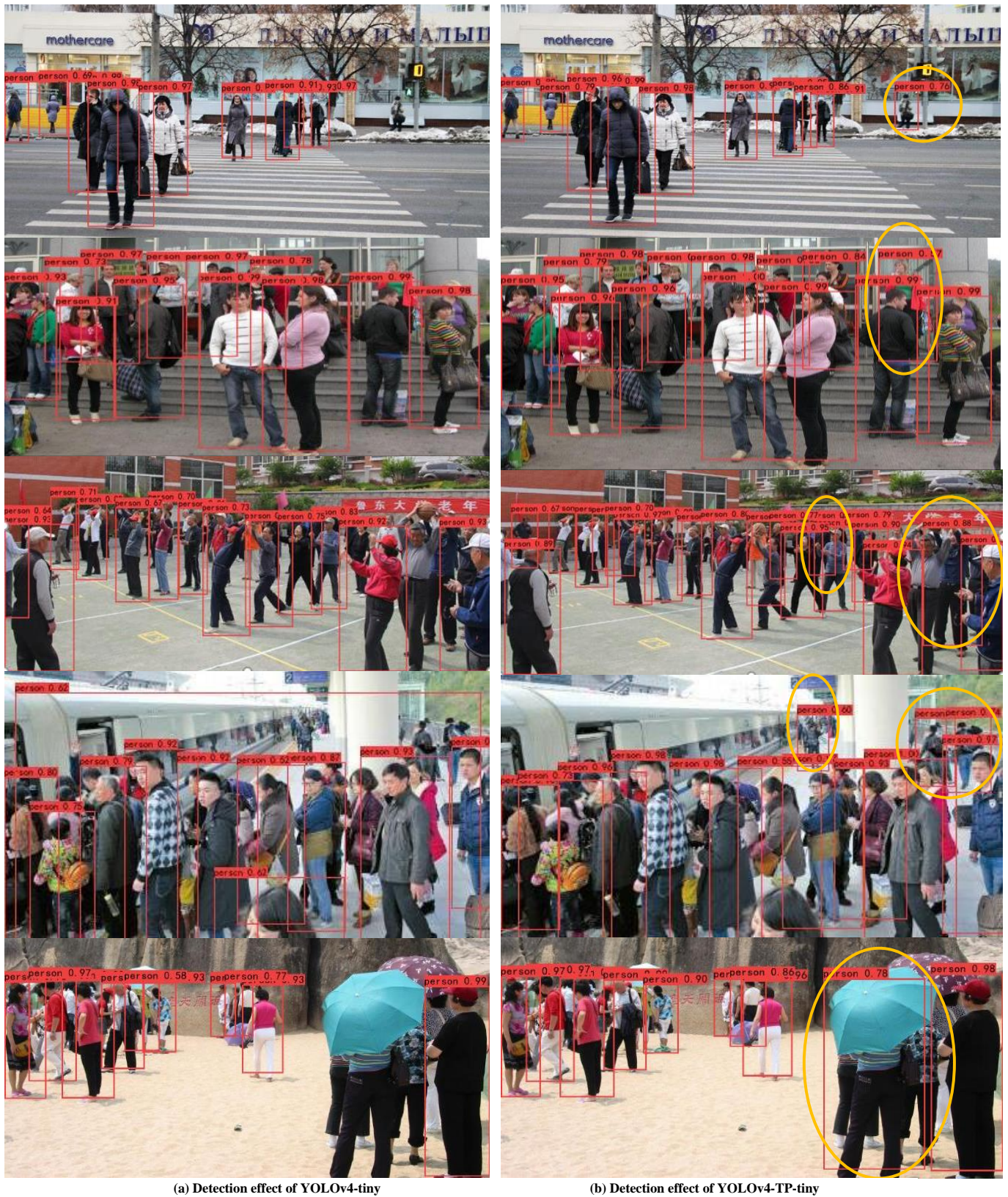
Figure 11. Comparison of detection effect between the YOLOv4-tiny and the YOLOv4-TP-tiny on the widerperson dataset.
