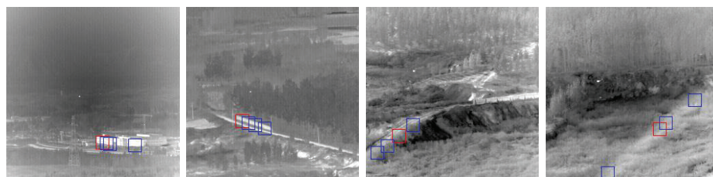
Figure 1. Illustration of matching blocks of infrared images. Each image shows a reference block marked with red borders and a few of the blocks marked with blue borders matched to it.
