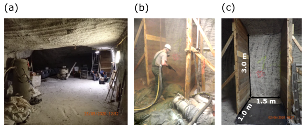
Figure 1. Impressions from shotcrete experiments at Teutschenthal mine: (a) experimental underground site, (b) during shotcrete procedure at a shotcrete box, (c) preparation of a shotcrete box.
