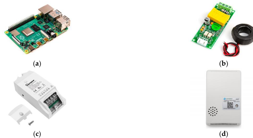
Figure 5. Selected devices for data acquisition layer: (a) Raspberry Pi 4B; (b) PZEM-004t-100 A; (c) Sonoff Pow R2; and (d) Air quality LAQ4.
