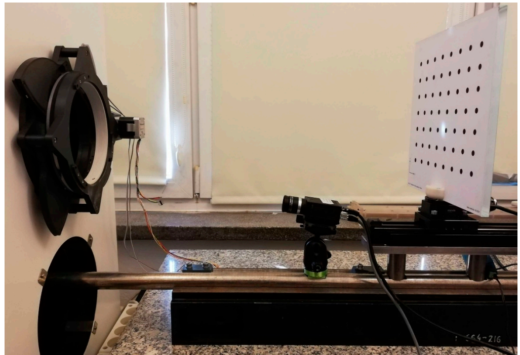
Figure 4. Photo of the test stand with the additional camera attached for the stability measurement. The light-emitting diode (LED) panels were temporarily removed for a better view of camera.
