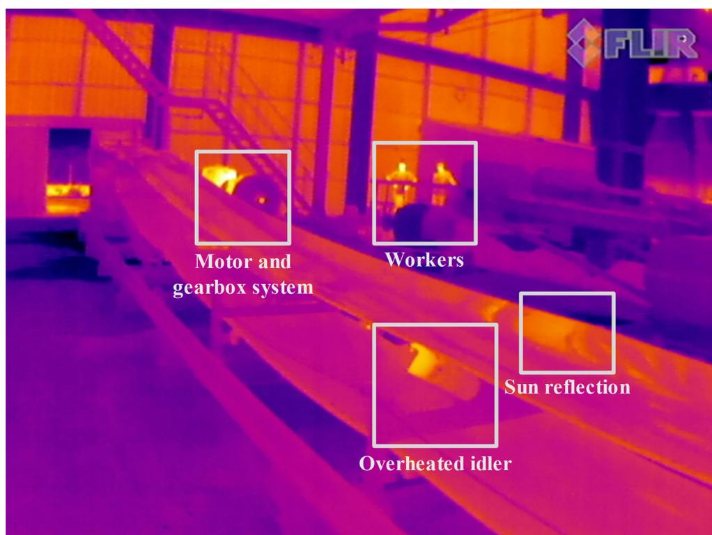
**Figure 6.** Examples of IR sources that are not related to idlers.
