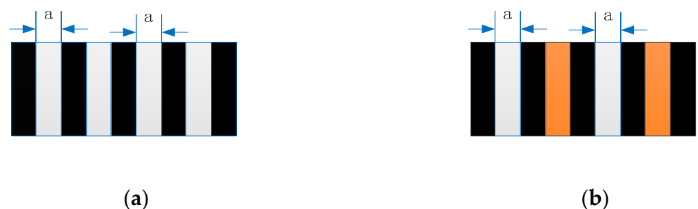
Figure 3. Different types of scanning reticles. (a) A traditional scanning reticle made by amplitude grating. (b) The proposed scanning reticle made by combination of amplitude and phase grating.
