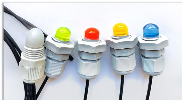
Figure 2. Series of fabricated luminescent sensor heads.
