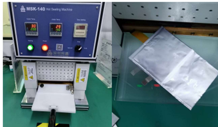
Figure 7. The optical photograph of the fabrication of the pouch cell embedded with the sensor array.
