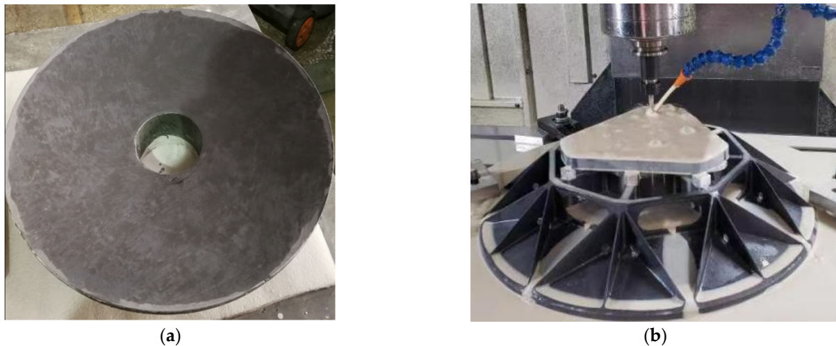
Figure 11. The primary mirror blank. (a) The front; (b) the back being machined.
