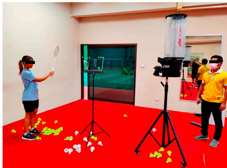
Figure 18. Effect of different string pattern, tension, diameter, and hitting reaction on a professional player (photo taken at Badminton Sport Center, Walailak University).
