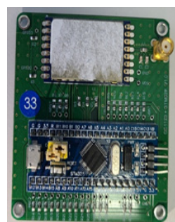
Figure 4. Transceiver configured with STM32F103 + CC1120.
