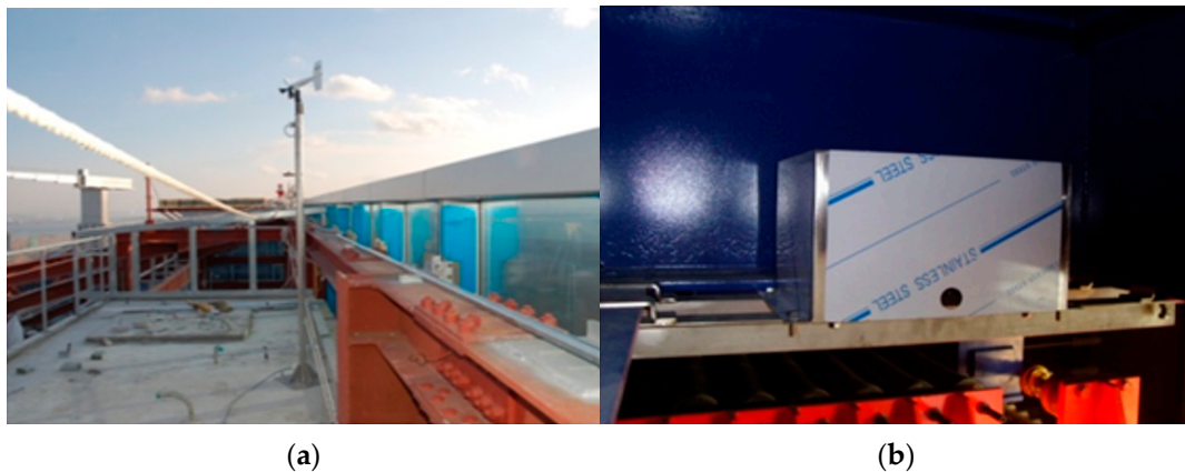
Figure 3. Data acquisition: (a) Anemometer on the top level of the tower; (b) the accelerometer installed on the TMD.
